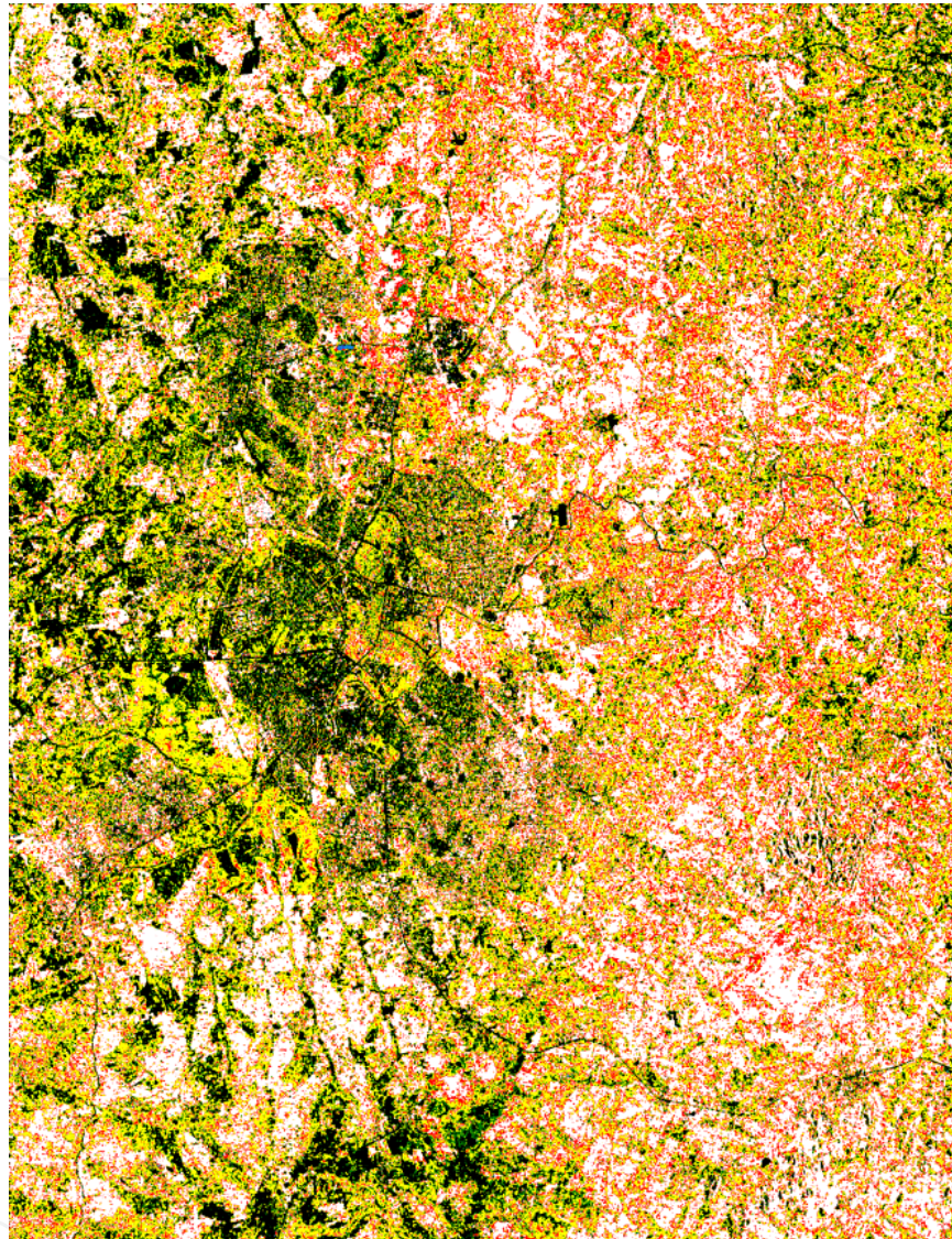
Figure 9. Result of combining the classification results of the two amplitude images from Figure 8 according to Table 1, where: L – black, C – blue, ML – green, M – yellow, MH – red, H – white.
