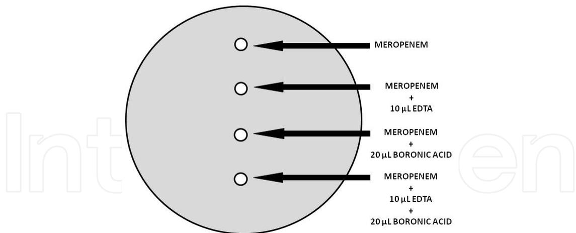
**Figure 9.** Preparation of the combination meropenem disc test.
