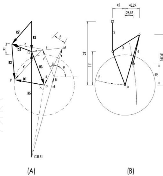
Figure 5. (A) Vector analysis used in the synthesis process of the climbing mechanism. (B) Resulting climbing mechanism
