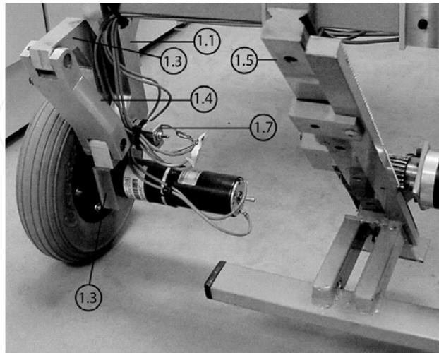
Figure 11. Details of the Climbing Mechanism
