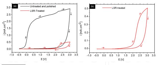
Reprinted from Applied Surface Science 2013, 276,1, Pariona MM, et al., Influence of laser surface treated on the characterization and corrosion behavior of Al–Fe aerospace alloys, Copyright (2013), with permission from Elsevier [License Number:3176530612877] [6].
