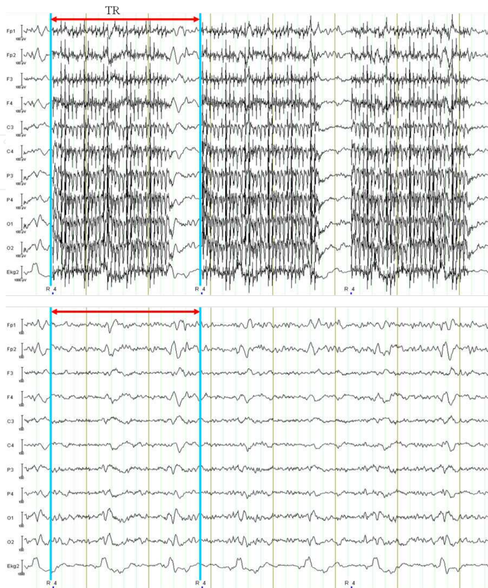
Figure 2. EEG signals recorded from 10 different channels (Fp1, Fp2, F3, F4, C3, C4, P3, P4, O1, O2) and ECG signal with the image acquisition artefact (top) and after the IAA reduction (bottom)
