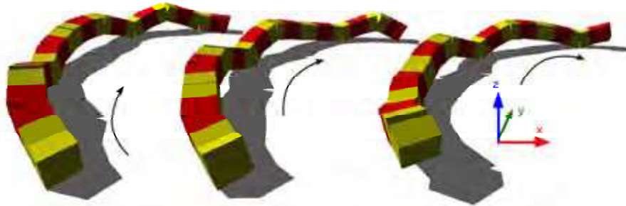
Figure 19. A pitch-yaw connecting modular robot performing the turning gait for k=3
