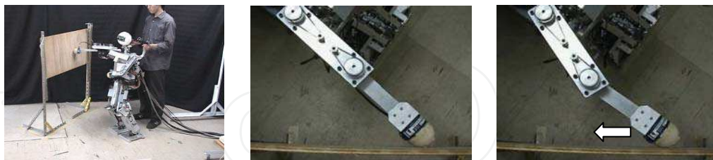
Fig. 2. Photographs of robot and robot's arm during groping on wall surface.
