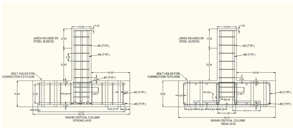
**Figure 6.** Elevation View of the Strong Axis of the Shear-Critical SCRC and SCCNFC Columns and Foundations (dimensions in inches)
