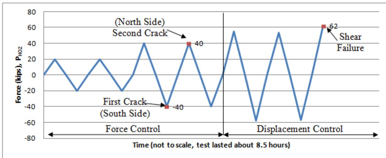
**Figure 9.** SCRC Column Load Path
