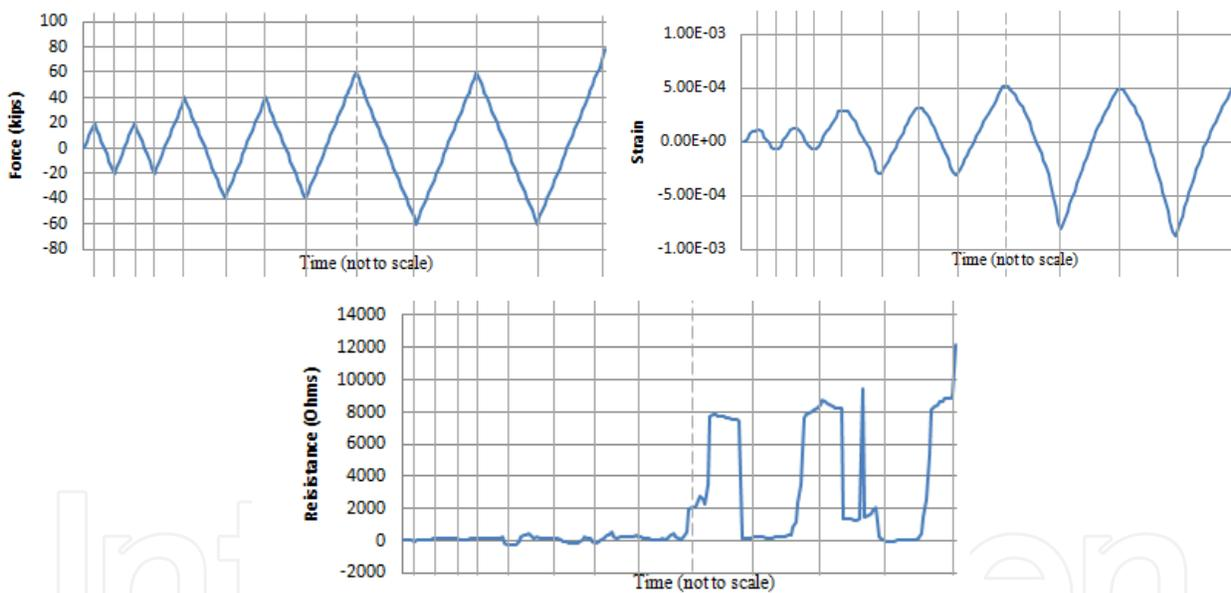
Figure 13. SCRC Column Comparison of Horizontal Force, LVDT Strain and Electrical Resistance on North Side
