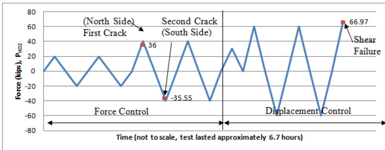
Figure 11. SCCNFC Column Load Path
