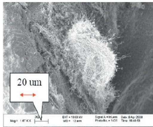
**Figure 2.** Scanning Electron Microscope Image of CNF Clump in Normal Cement (1670x Magnification)
