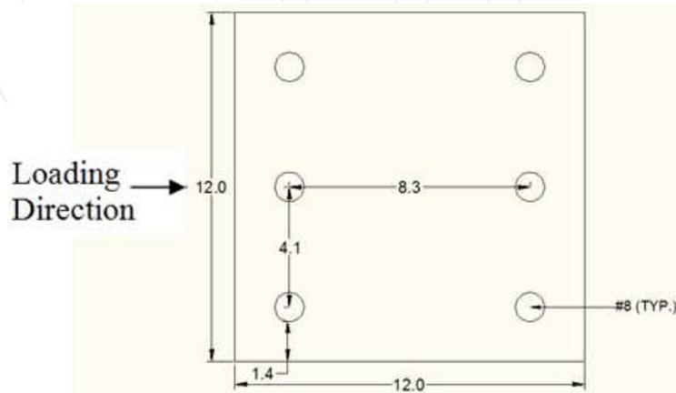
Figure 5. Cross-Section of SCSFC Column (dimensions in inches)
