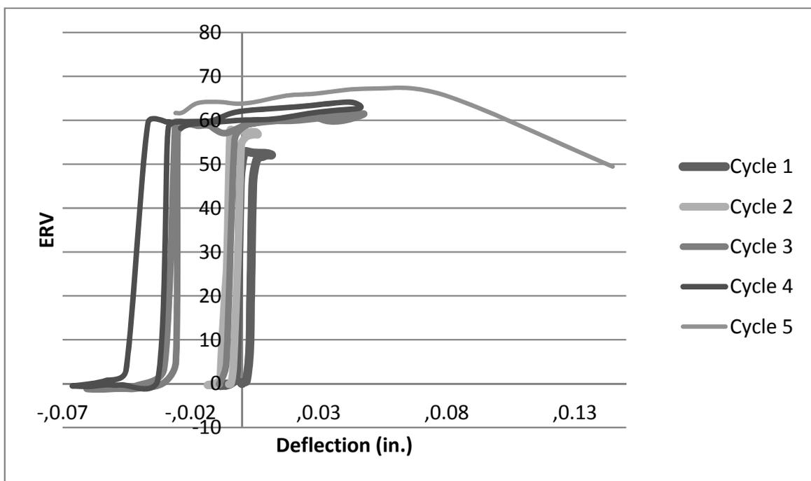
**Figure 15.** SCCNFC Column ERV versus Horizontal Deflection
