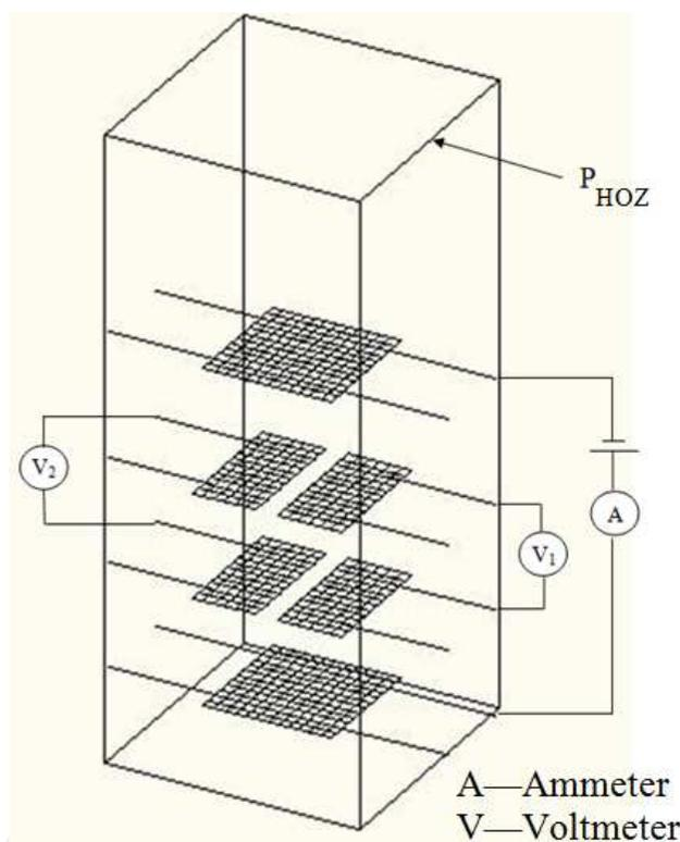
**Figure 8.** Four Probe Method of Resistance Measurement
