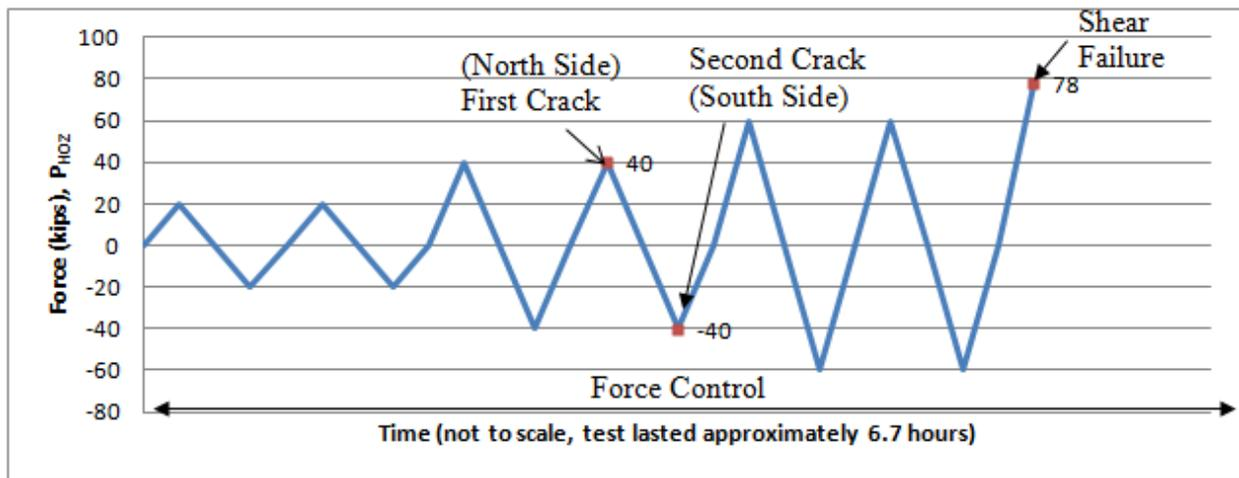
Figure 10. SCSFC Column Load Path
