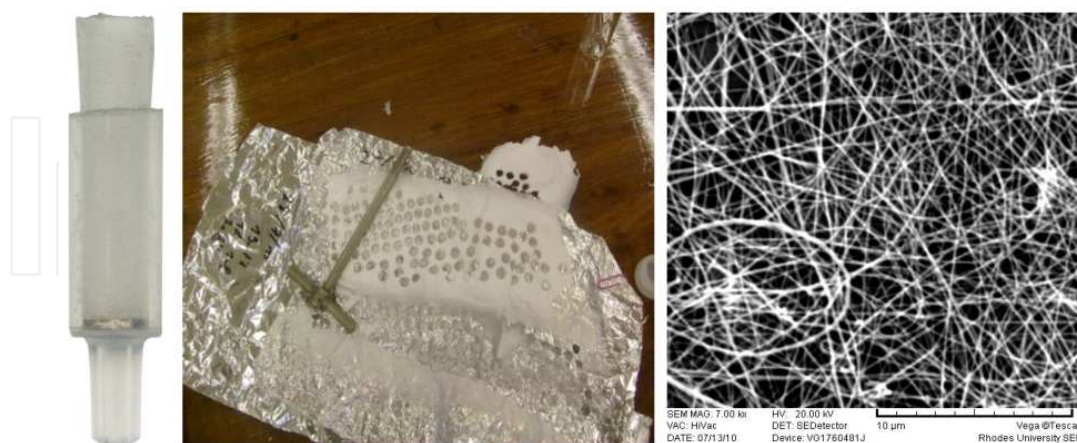
Figure 13. (a) Photograph of disk (II) SPE device, (b) photograph of an electrospun nylon 6 nanofiber mat showing regions from which disks were cut and (c) SEM image of sorbent bed zoomed in top surface [59].
