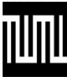
Figure 21. Structure of delaying line converters
