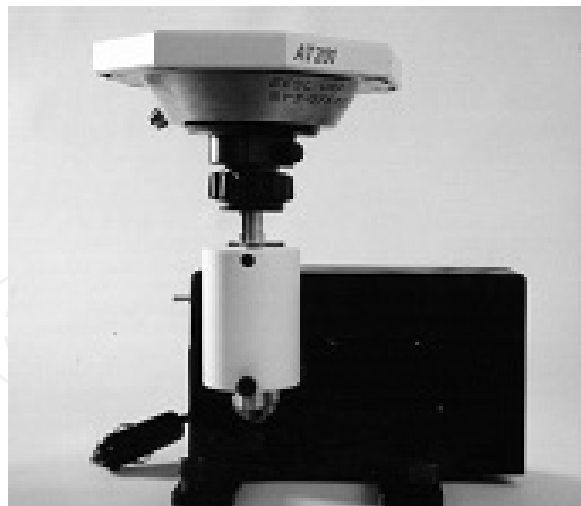
Figure 7. GPS antenna over the electro-mechanical oscillator
