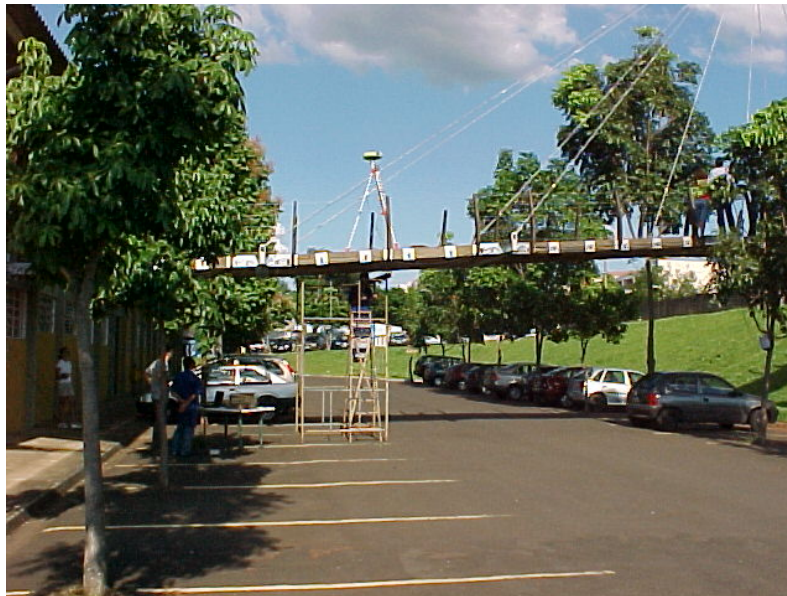
Figure 13. The GPS receiver and transducer of displacement installed in a footbridge
