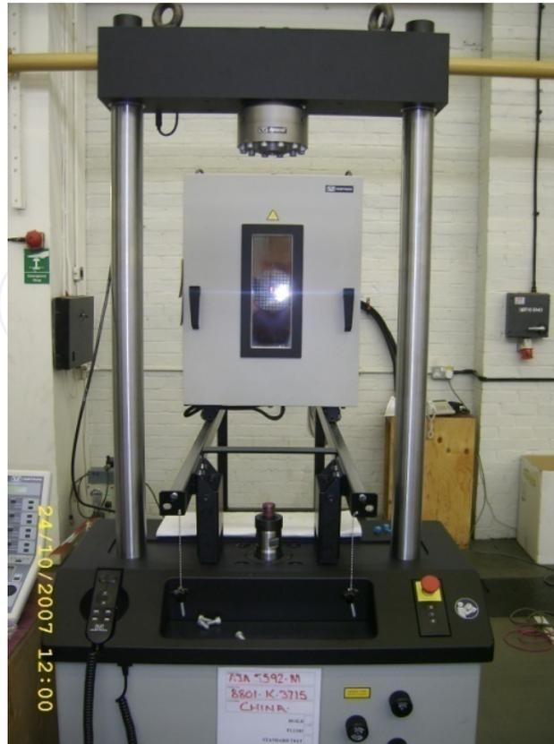
**Figure 5.** Temperature chamber mounted to 8872 Instron machine (High Wycombe)
