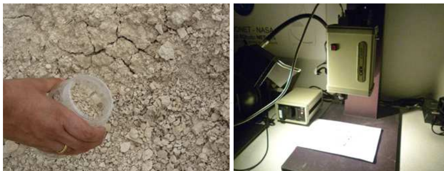
Figure 2. Collection of soil data (left). Spectroradiometric measurements of material samples at the premises of the Remote Sensing and Geomatics Laboratory of CUT (right)
