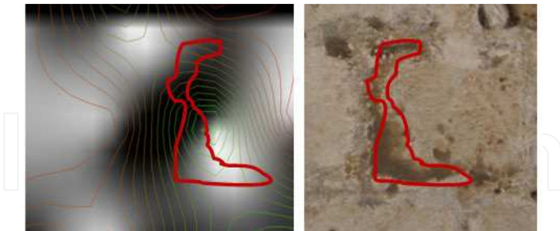
Figure 24. Visual comparison of the ultrasonic measurements and close range photographs. The polygons are drawn as common areas for each set of figures.
