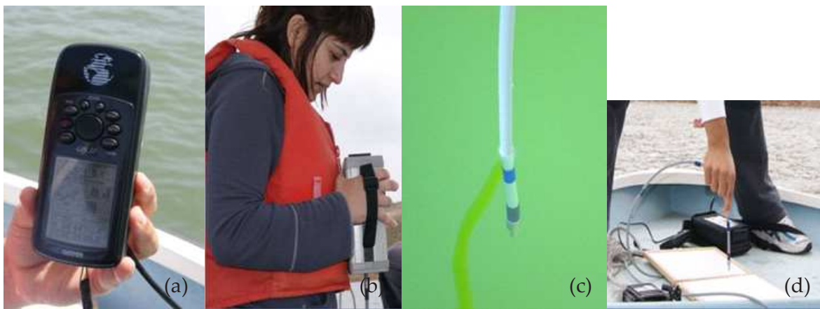
Figure 6. Equipments used during field campaigns (a) Global Position System Garmin GPS72; (b) handheld GER-1500 field spectroradiometer; (c) fibre optic probe & (d) standard Spectralon panel.
