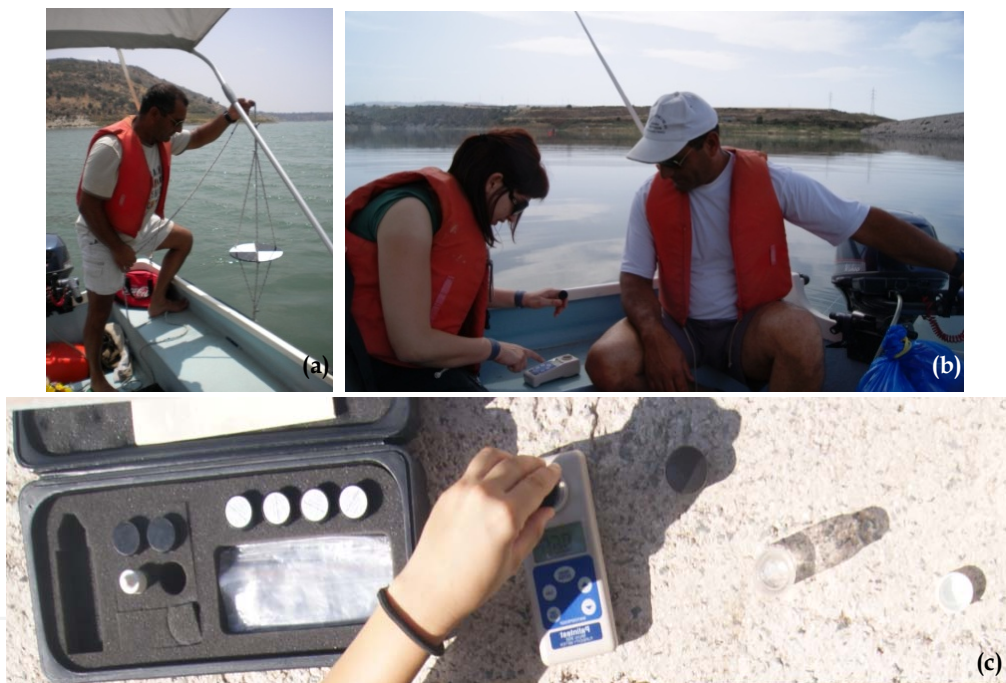
Figure 7. Measuring the turbidity in Asprokremmos Dam using both (a) the Secchi Disk and (b&c) the portable turbidity meter; Palintest Micro950.
