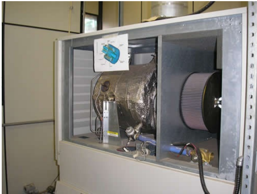
Figure 7. Capstone microturbine in the laboratory at UNIFEI.
