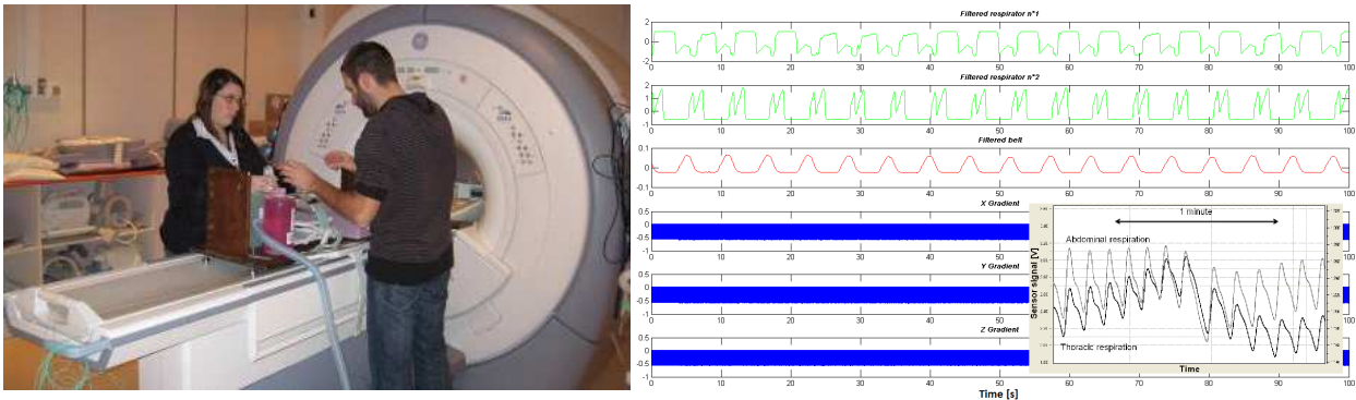
Figure 26. Left: Set-up of the MRI-compatible simulator of CIC-IT de Nancy, France. Right, large picture: Test of the FBG sensor in MRI environment. The first two curves are related to the respiration simulator, the third curve shows the FBG sensor response and the last three curves are related to the magnetic gradients of the MRI equipment. Right, small picture: Abdominal and thoracic respiration signals detected by the textile-embedded macrobending and FBG sensor during a clinical test on healthy volunteers.
