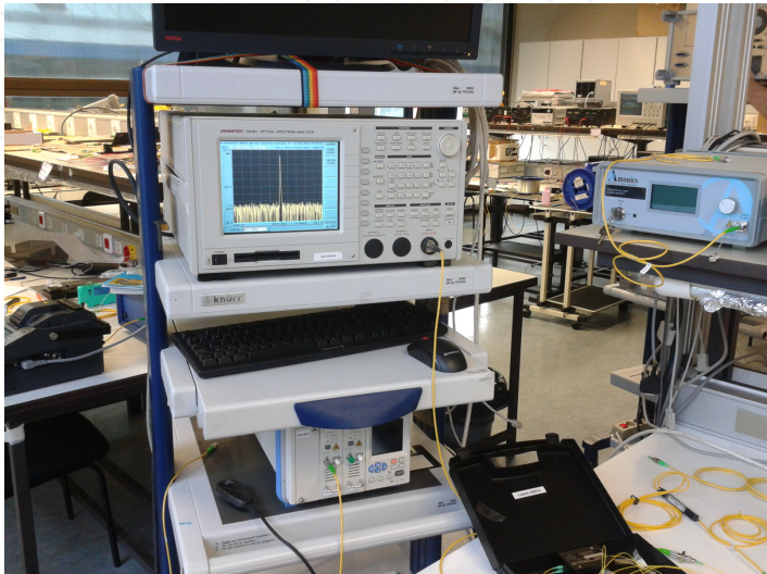
Figure 2. Experimental setup of a short-cavity fiber laser
