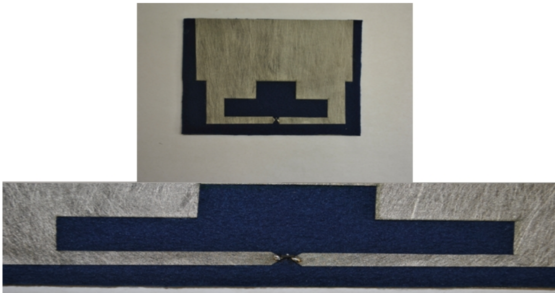
Figure 28. Fabrication and Chip connection for TAG 3
