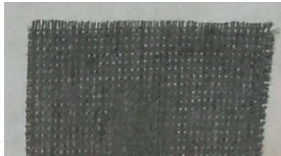
Figure 9. Photo of woven Betex textile material
