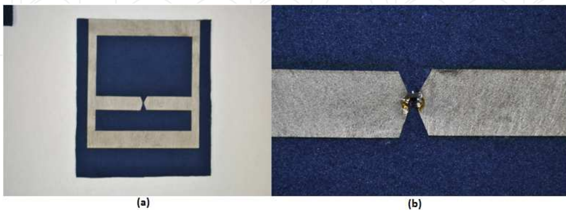
Figure 26. Fabricated antenna (a), chip connection to slot arm (b) for TAG 1
