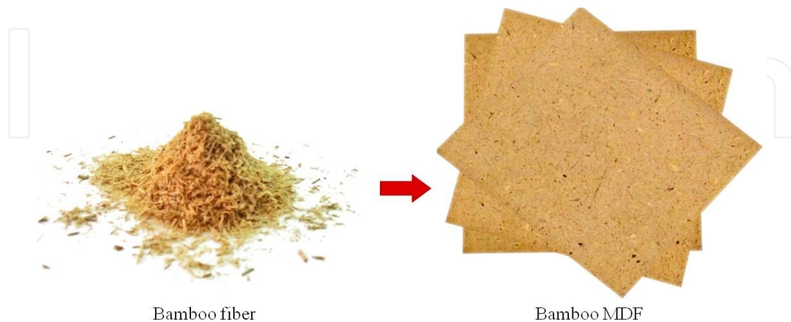
Figure 4. Bamboo Medium Density Fibreboard (MDF) from bamboo fibre.
