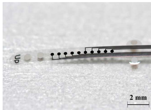
Figure 10. Parylene MEA for murine spinal cord stimulation and recording.
