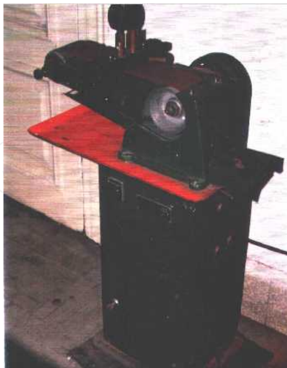
Figure 2. The pin-abrasion testing machine [19, 20]
