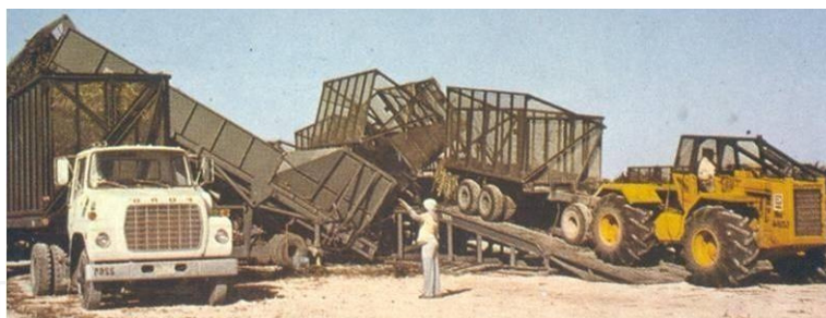
Figure 2. Transfer of sugar cane from in-field hauling trailers to highway-hauling trucks.
