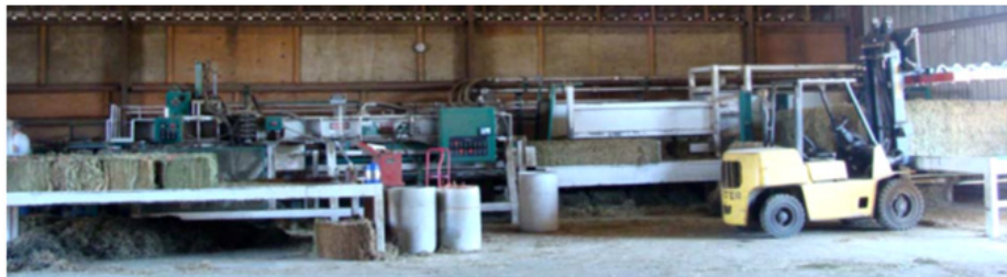
Figure 4. Commercial large rectangular bale slicer/compressor.
