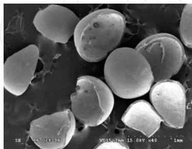
Figure 8. Appearances of SiC coating layer after crushing
