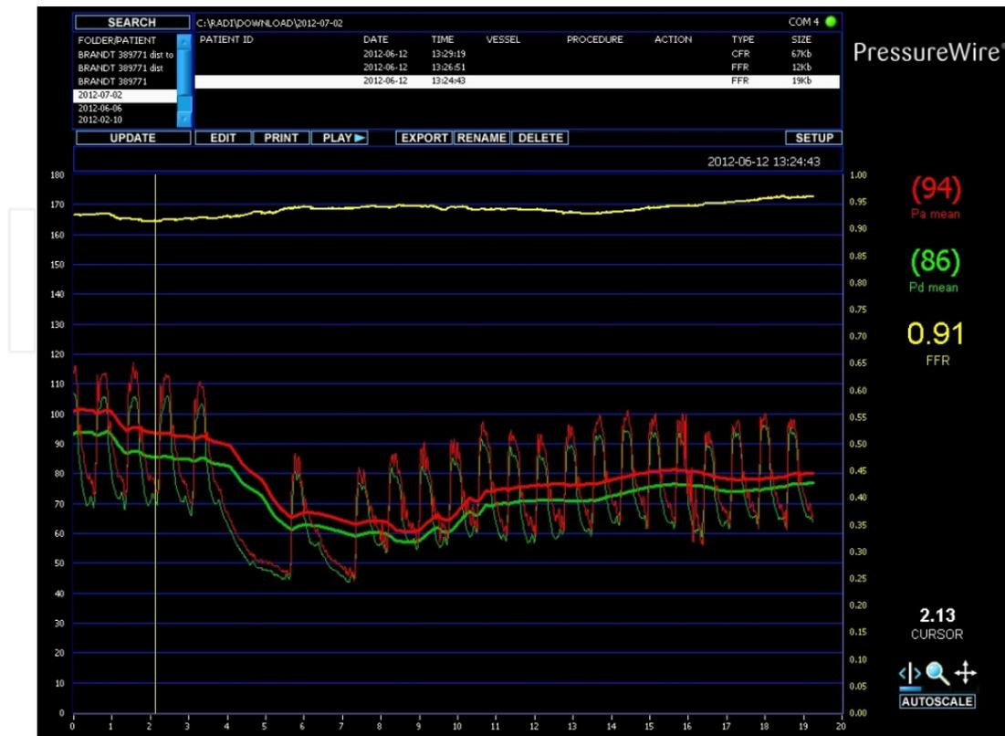
**Figure 1.** Typical Example of FFR Recording (n.b. mean Pd and Pa pressures and automatic FFR recording as well as transient bradycardia consistent with adenosine)
