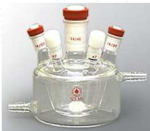
Figure 1. Electrochemical cell used for cyclic voltammetry experiments.
