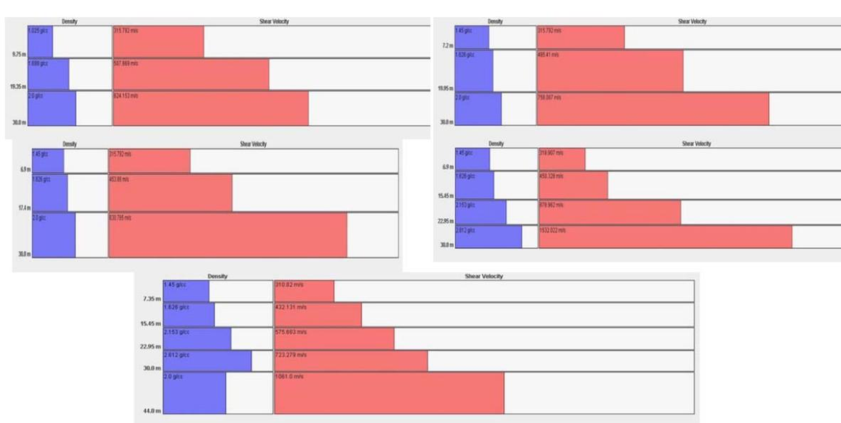
Figure 12. Shear wave velocity model calculated for refraction microtremors profiles ReMi-1 To ReMi-5 (Figure 9).
