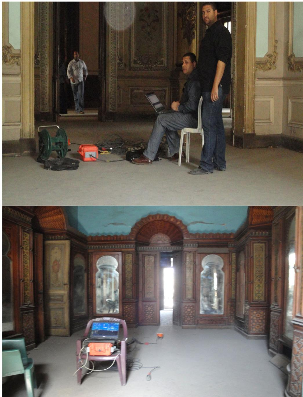
**Figure 20.** High dynamic range ES-3000 Geometrics mobile station and triaxial geophone used 4 Hz to drive structure response of El-Sakakini Palace.
