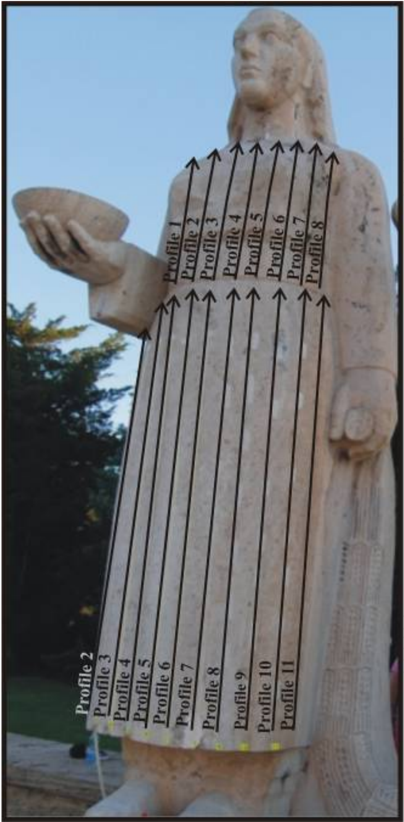
Figure 5. GPR data acquisition scheme of the first female statue.
