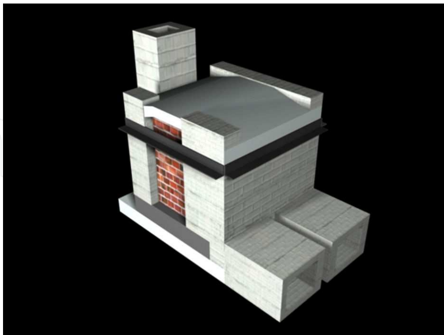
Figure 8. A typical model of a kiln design constructed for the purpose of ceramic firing research (Adelabu O.S, 2011).
