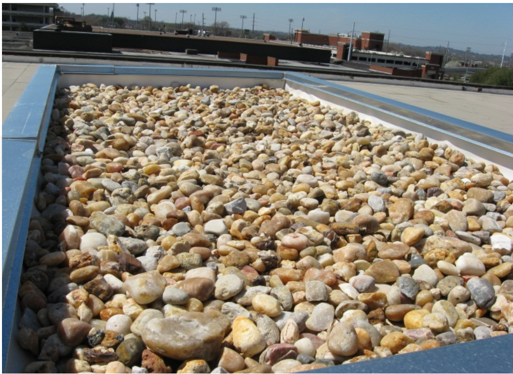
Figure 7. Mini-roof equipped with river rocks.
