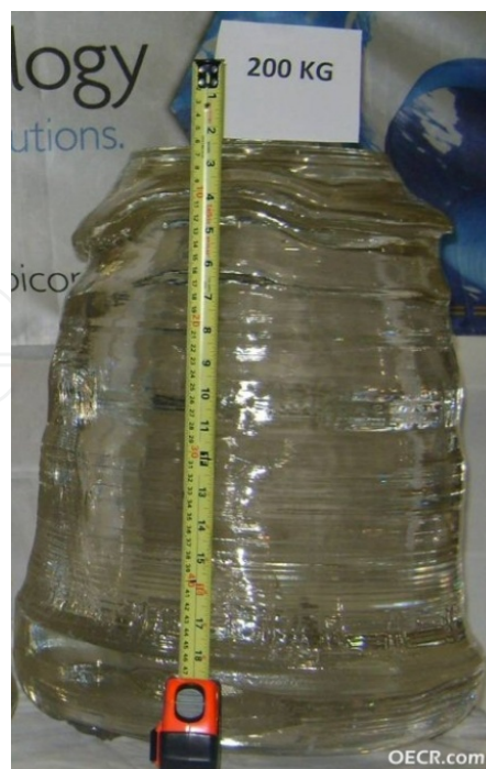
Figure 9. Sapphire boule grown by Rubicon Technology Inc.[17].
