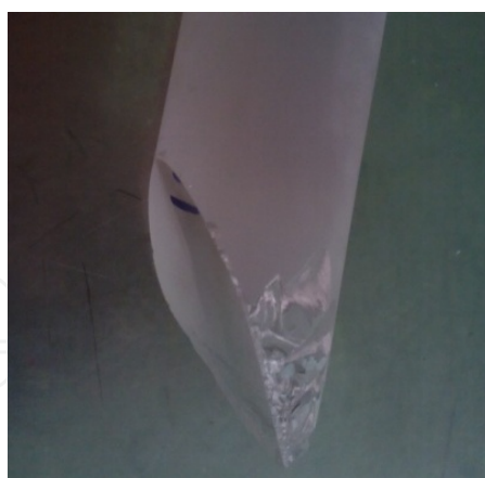
Figure 27. Cracking in the sapphire rod with stress.
