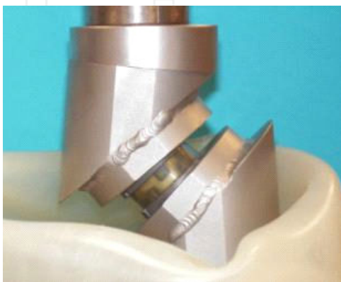
Figure 10. Wear tests were conducted in a 3-axis motion simulator (frequency = 4 Hz, loads of 135 to 1350 N), The inclination of the prosthesis was 45° to reproduce the sagittal orientation of the disk in functional situations. The gap between the metal plates was measured after each series of 10 million cycles.
