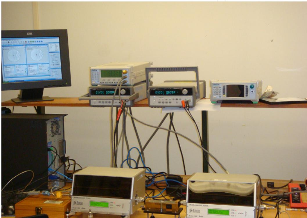
Figure 10. Load-pull bench used to characterize the device
