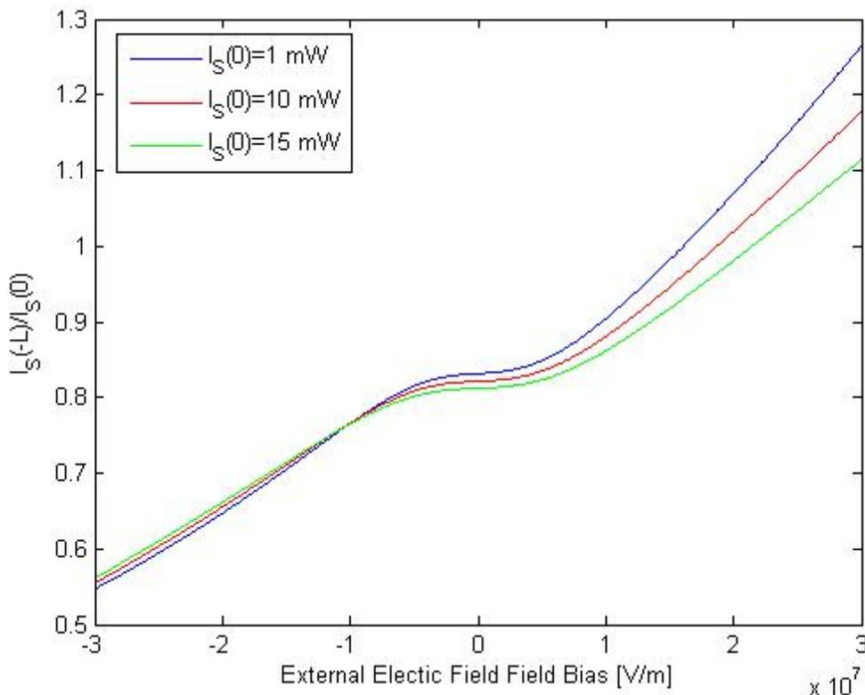
**Figure 7.** Net signal gain in electrically induced photorefractive silicon waveguide
