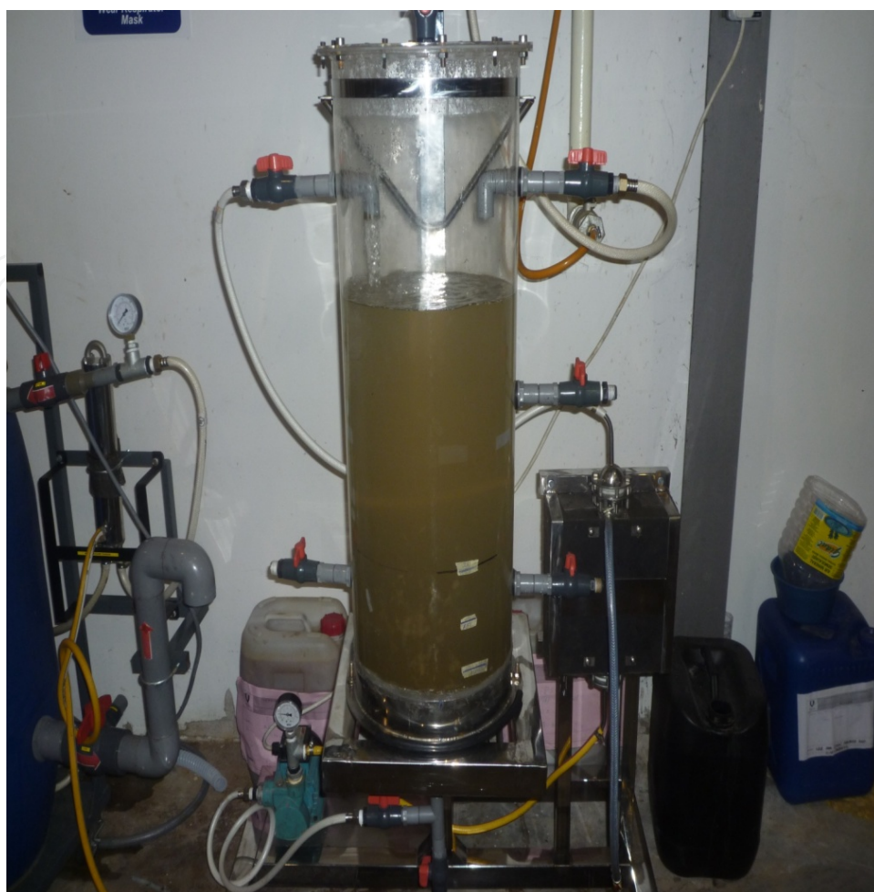
Figure 2. Schematic for Ultrasonicated membrane anaerobic system (UMAS)
