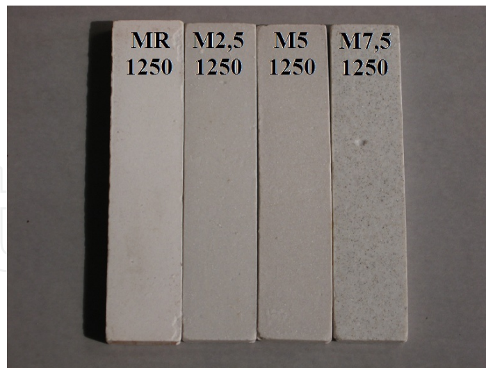
Figure 13. Appearance of the floor tile pieces after sintering.
