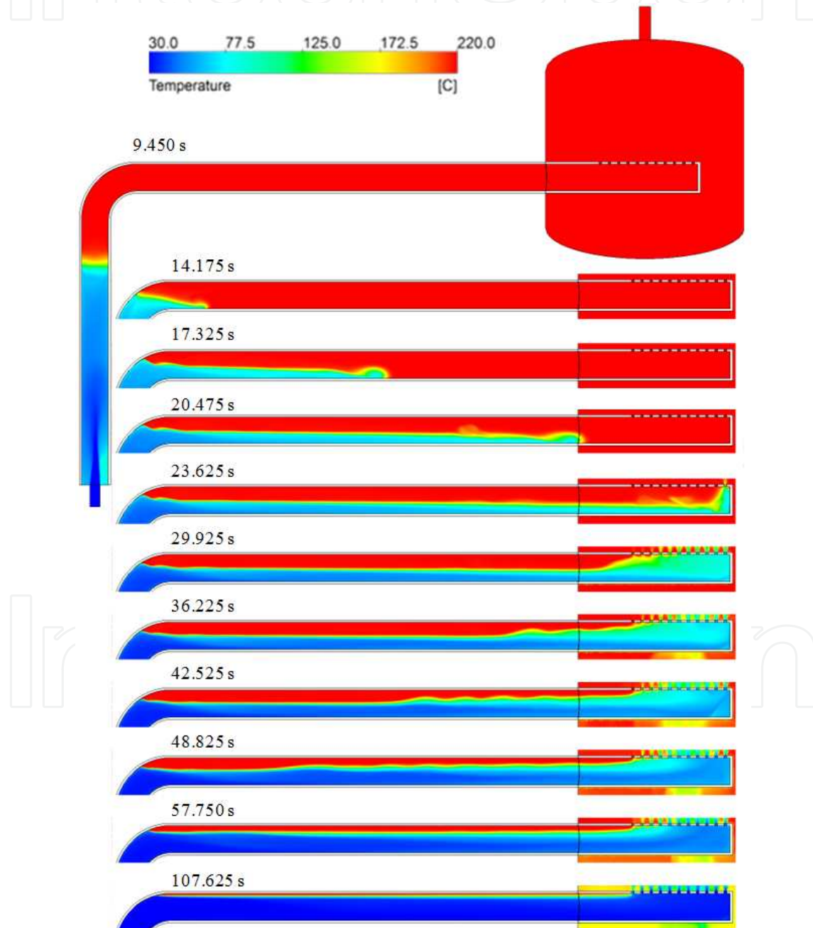
Figure 17. Temperature contours along time for flow rate 1.12 kg/s.
