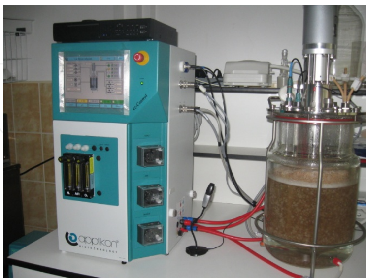
Figure 1. Laboratory-scale bioreactor for submerged cultivation of edible and medicinal mushrooms
