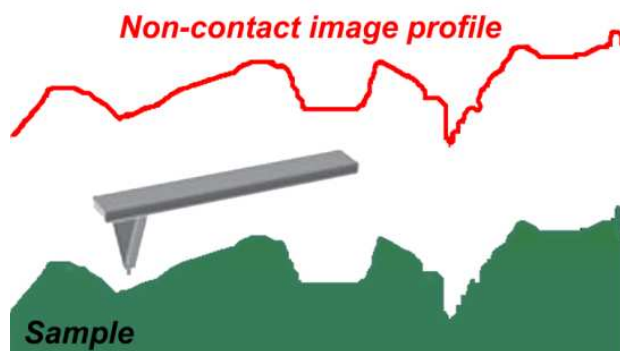
Figure 4. Schematical depiction of the non-contact AFM mode.
