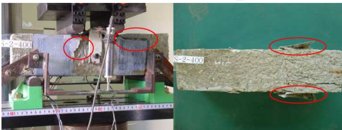
Figure 3. De-lamination of CFRP at failure
