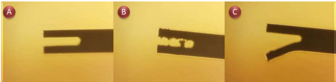
Figure 3. Magnified view of FP1NS50H pins (V&P Scientific, Inc.) with A) clean slot B) dirty slot C) damaged slot.
