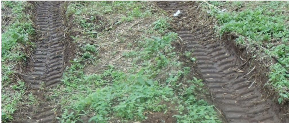
Figure 7. Plan view of the rut produced by the excavator tracks during experimentation
