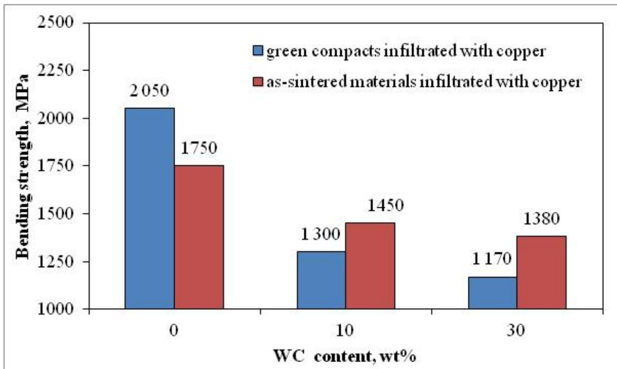
Figure 12. The Bending Strength of as-infiltrated composites
