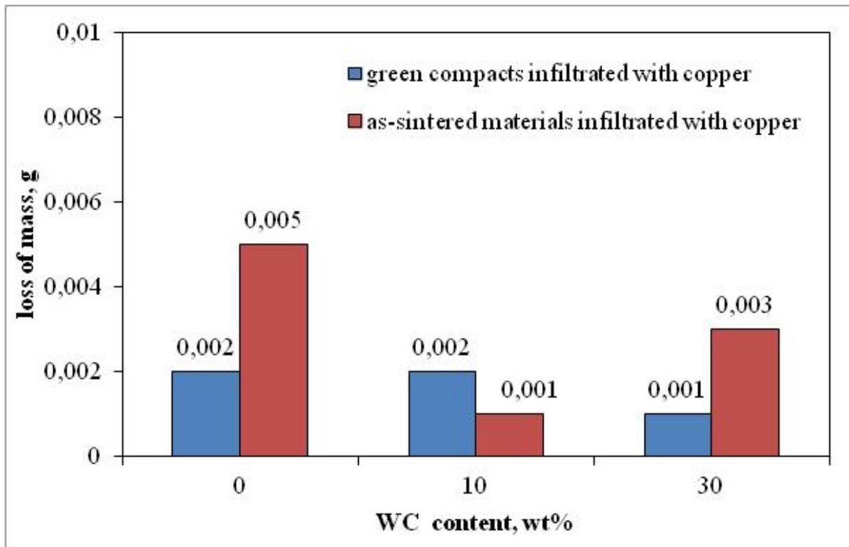
Figure 23. Loss of mass of as infiltrated composites
