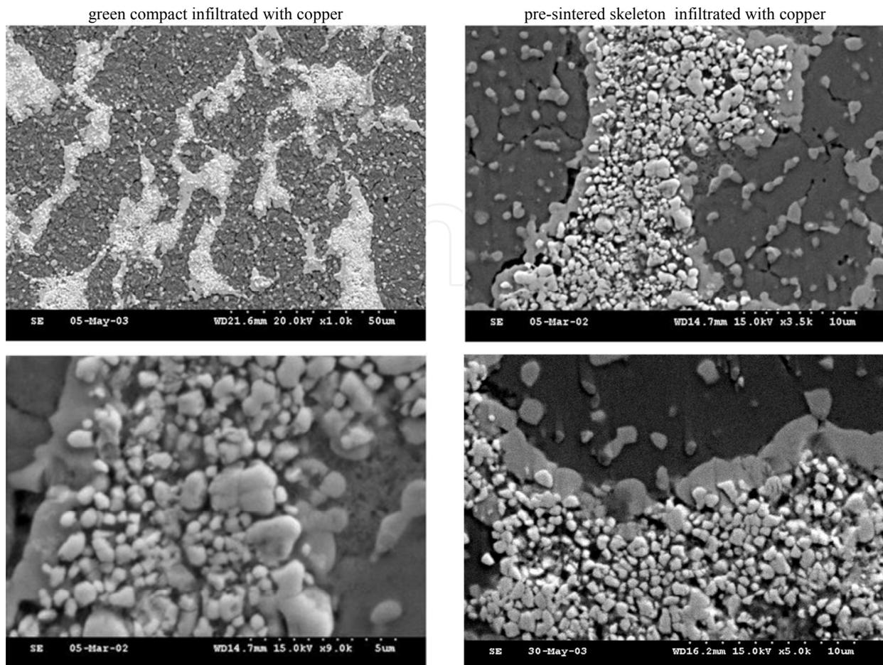
Figure 17. SEM microstructures of M3/2 HSS + 30%WC composites
