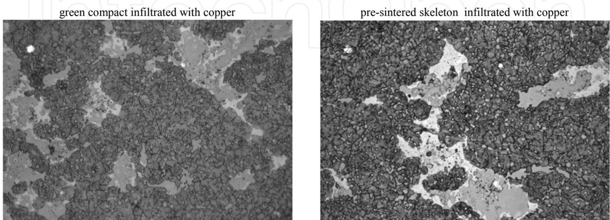
**Figure 14.** Microstructures of M3/2 HSS + 10%WC composites
