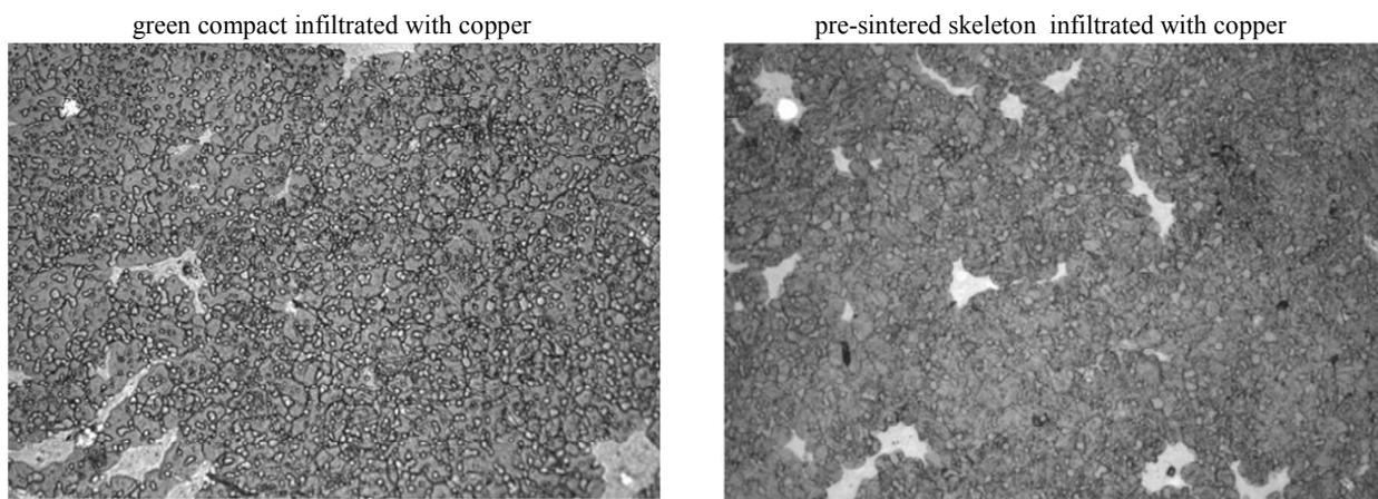
**Figure 13.** Microstructures of M3/2 HSS based composites
