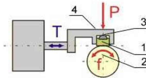
**Figure 3.** Tribosystem T05 - wear test principle
