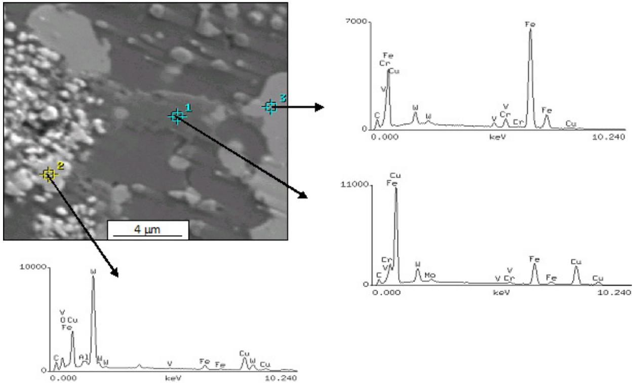
**Figure 20.** The microstructure of pre-sintered skeleton M3/2+30%WC infiltrated of copper and the qualitative EDX analysis, 1 – steel matrix, 2 – tungsten carbide WC, 3 – carbide M<sub>6</sub>C type
