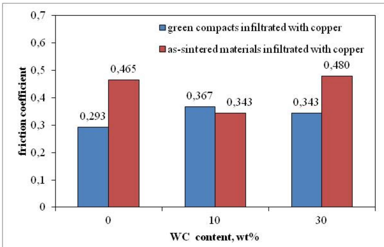
Figure 24. Friction coefficient of as infiltrated composites
