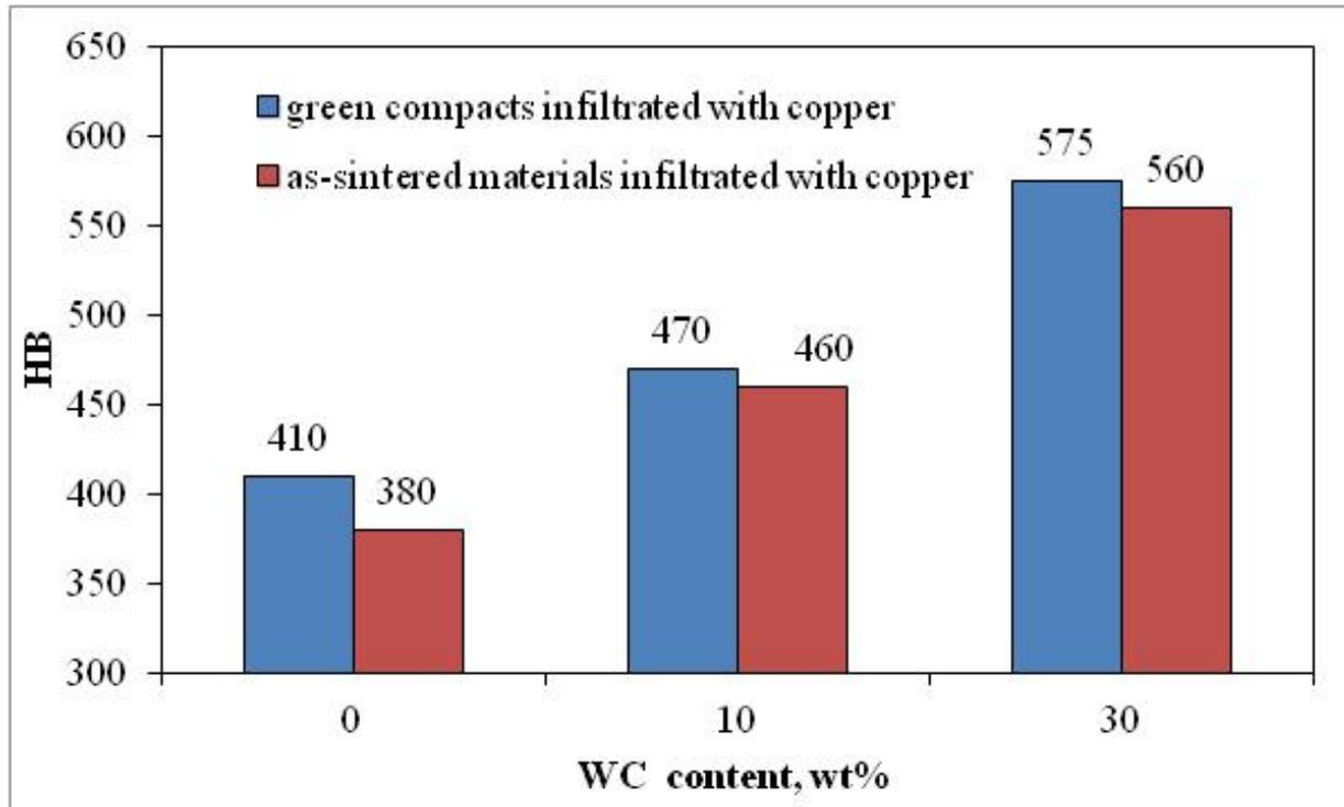
Figure 11. The Brinell Hardness of as-infiltrated composites
