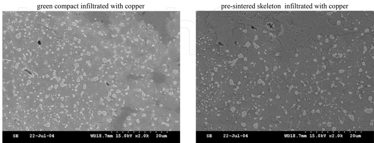
**Figure 16.** SEM microstructures of M3/2 HSS based composites
