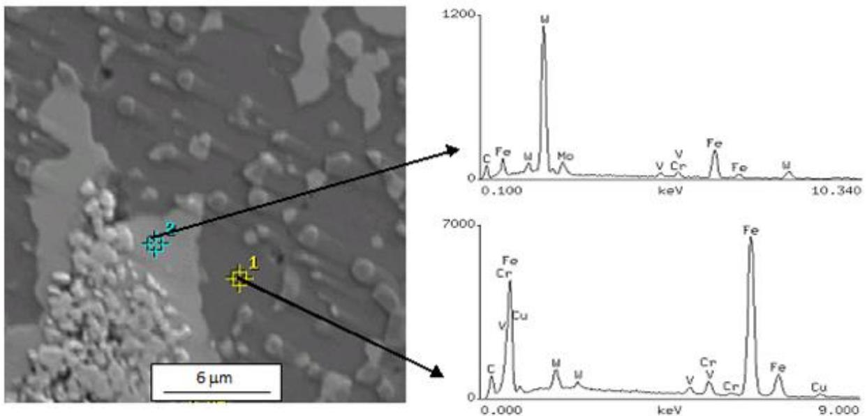
**Figure 21.** The microstructure of pre-sintered skeleton M3/2+30%WC infiltrated of copper and the qualitative EDX analysis, 1 – steel matrix, 2 – carbide M<sub>6</sub>C type
