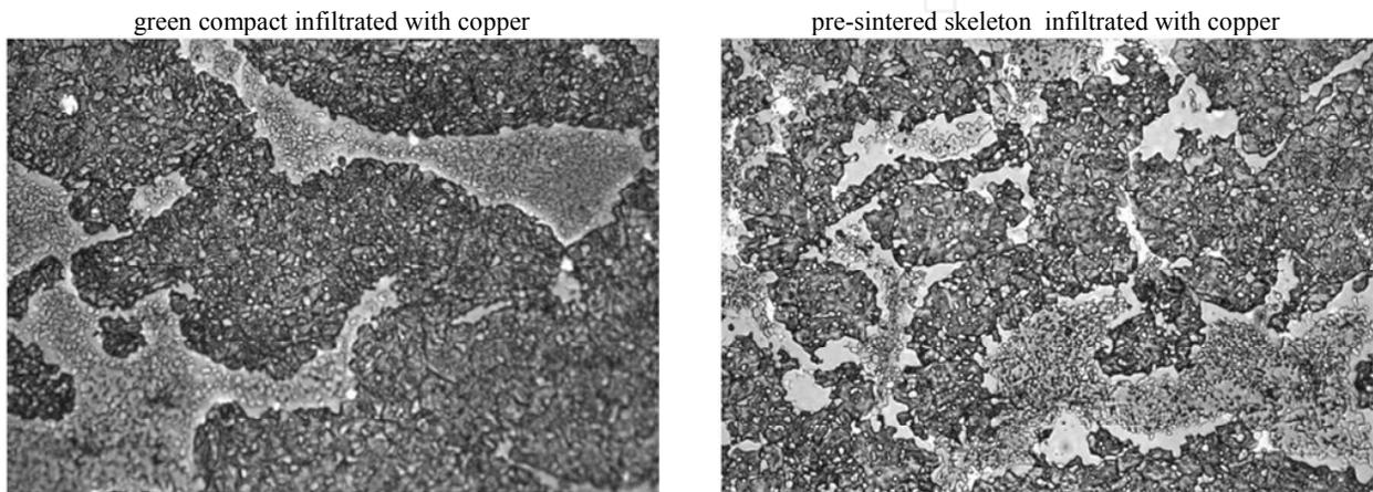
**Figure 15.** Microstructures of M3/2 HSS + 30%WC composites
