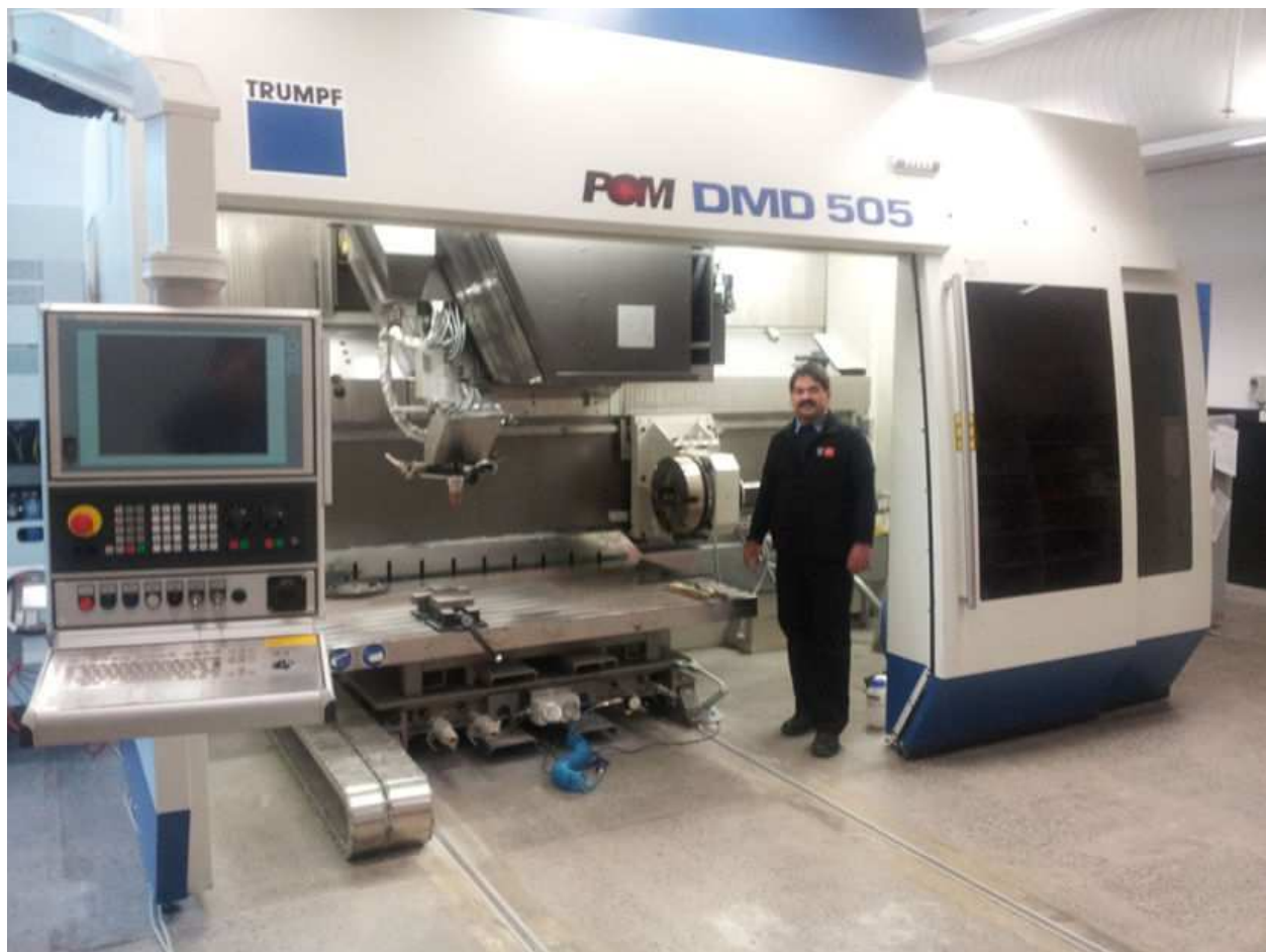
Figure 1. POM DMD (direct metal deposition machine) featuring 6-axis rotating, CAD-CNC control using a 5kW CO 2 Trumf laser.
