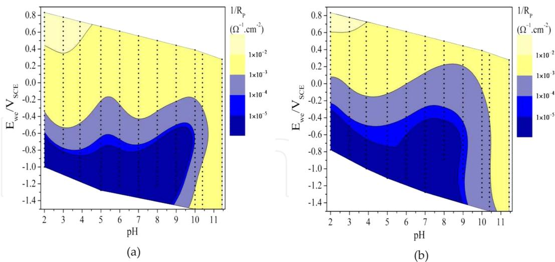
**Figure 4.** Contour plots of  $1/R_p$  for the E-pH space and their data for (a) A portion of a 99.9999% Al ingot single crystal and (b) a polycrystalline specimen from the identical ingot in (a) (adapted from (Zhou, Birbilis et al. 2010)
