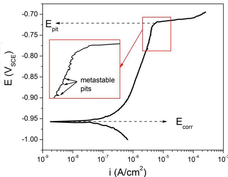
**Figure 11.** Polarisation curve indicating the corrosion potential  $E_{\text{corr}}$  and  $E_{\text{pit}}$  with metastable pits region prior to  $E_{\text{pit}}$  highlighted in the inset (adapted from (Cavanaugh 2009))
