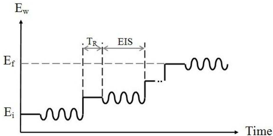
**Figure 10.** Illustration of polarizing signal during SPEIS
