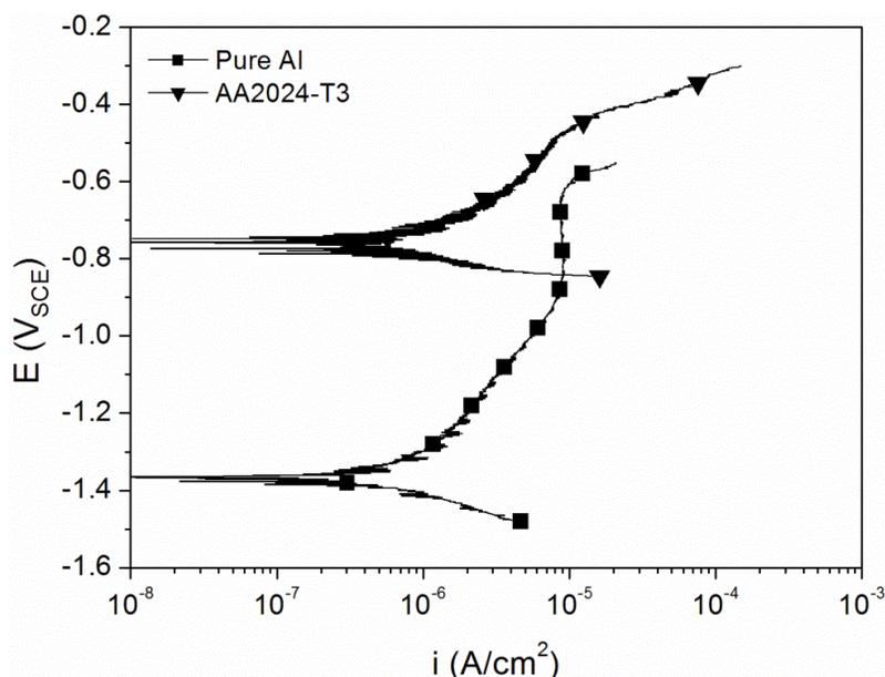
**Figure 3.** Polarisation curve of pure Al and AA2024-T3 exposed to 0.1M NaCl for 7 days collected at 1mV/s<sup>-1</sup> (adapted from (Sukiman, Birbilis et al. 2010))
