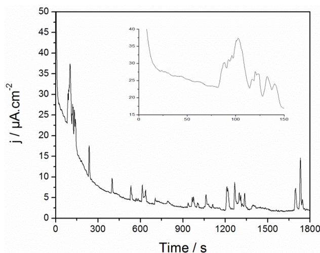
**Figure 12.** Current transient for AA5083-H116 obtained at 25mV below  $E_{pit}$ . Inset shows a zoom of a region of interest that represents the typical transient features (adapted from(Gupta, Sukiman et al. 2012))
