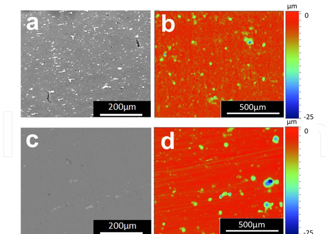
**Figure 6.** SEM images for AA2024-T3 and AA5083-H116 before exposure in (a) and (c) and after exposure in 0.1M NaCl for 14 days in (b) and (d). These are comparative images to show the extent of damage following immersion.
