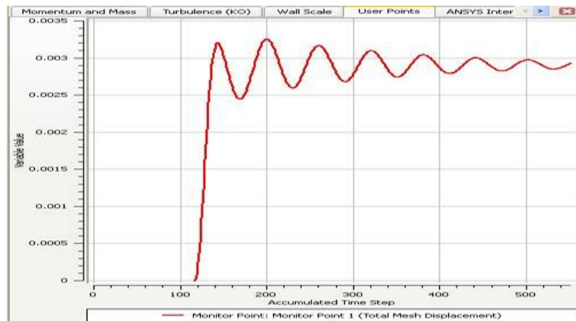
Figure 27. Oscillatory response to sudden subject to a constant flow of 15m/s
