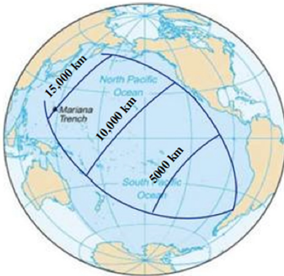
Figure 4. Propagation geometry of 1960 Chilean tsunami in a lune of angle 90^\circ with wavefronts at intervals of 5,000 km
