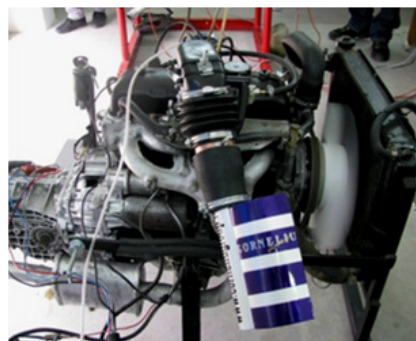
Figure 48. Supliform super absorbing filter trial
