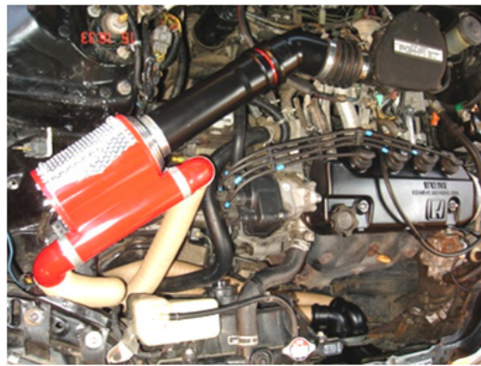
Figure 27. DATD, bi-route mounted on Honda Civic, 1.6
