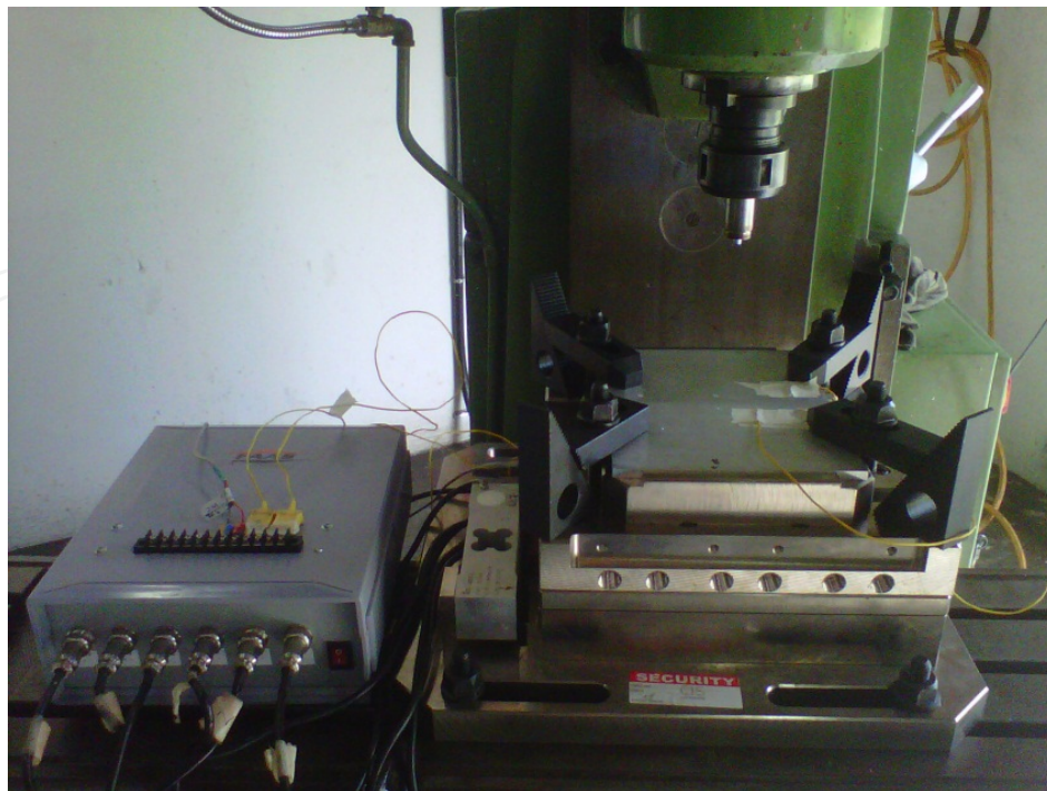
Figure 1. Friction stir welding experimental set up [5].
