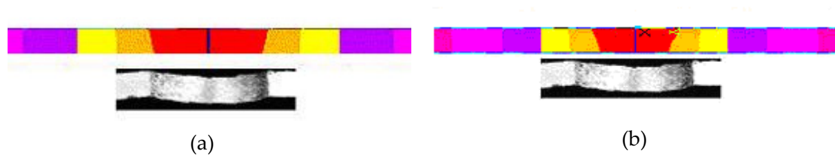
Figure 12. Experimental & simulated fusion boundary fitting: (a) double ellipsoid; (b) gaussian distribution;
